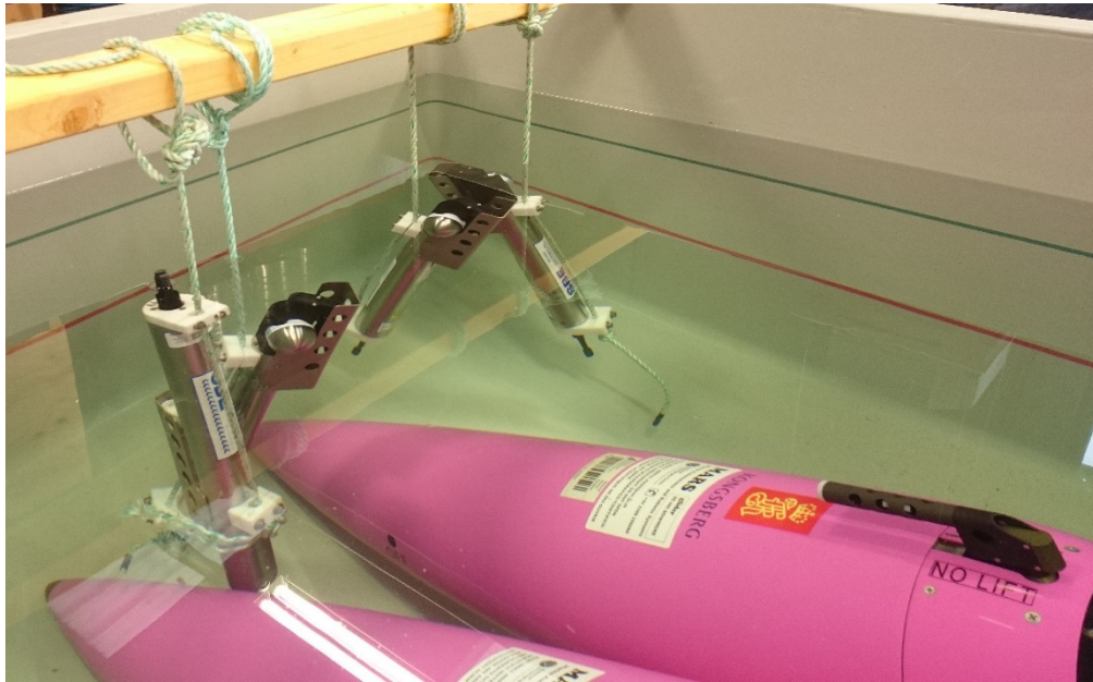
CAPTION: Testing new oxygen sensors (combined with sensors to measure temperature, salinity and pressure) at SAMS' Scottish Marine Robotics Facility, alongside two of its gliders ©Estelle Dumont.
